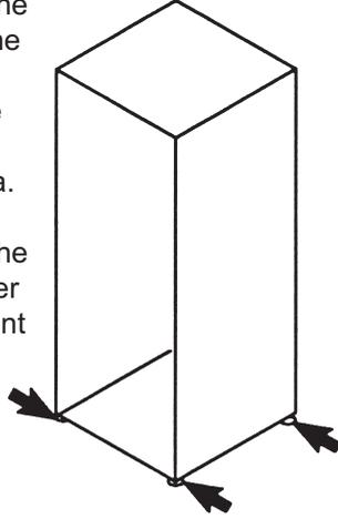
2. Adjust the levelers on one side until the front edges of the cabinet side panels are plumb (side-to-side).
