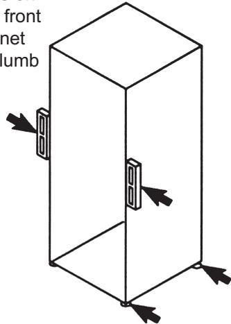
3. Measure A and B with a tape and adjust the front levelers until  $A=B$  ( $+1/32$  inch).
