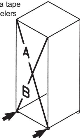
4. Adjust both front levelers equally until the front edges of the cabinet are plumb (front-to-back).
